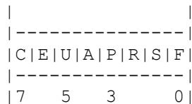
These are the TCP control bits we are interested in. We have numbered the bits in this octet from 0 to 7, right to left, so the PSH bit is bit number 3, while the URG bit is number 5.
