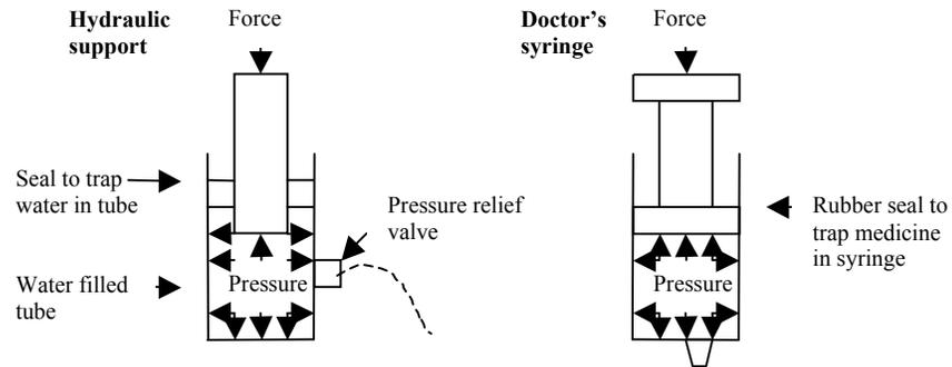
Therefore ‘hydraulic supports’ (hydro = water) use the principles of force and pressure such that as a force is exerted on the support, the water pressure increases. A pressure relief valve then squirts out water when the pressure (and thus the force) gets too large. Imagine a very large, modified doctor’s syringe.
