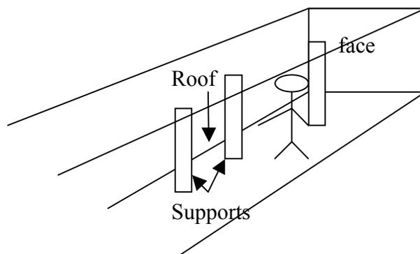
The roof is not one big uniform chunk of rock. Rather it is broken up into smaller chunks. It is assumed that the biggest chunk of rock in the roof has a mass of less than 20 000 kgs
