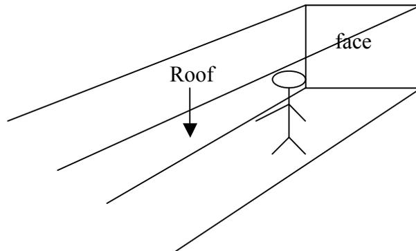
As one can imagine, a roof falling on one's head is not a nice prospect! Therefore the roof needs to be supported.
