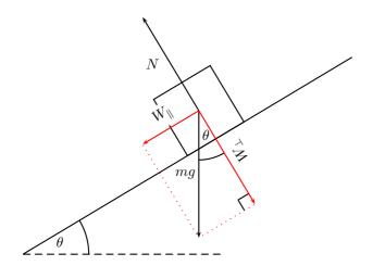
Now the object's weight can be resolved into components parallel and perpendicular to the inclined surface. These components are shown as red arrows in the diagram above and are at right angles to each other. The components have been drawn acting from the same point. Applying the parallelogram method, the two components of the block's weight sum to the weight vector.
