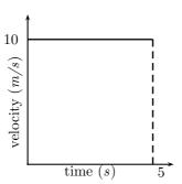
This graph shows an object moving at a constant velocity of 10m/s for a duration of 5s. The area between the graph and the time axis (the (NOTE TO SELF: SHADED) area) of the above plot will give us the displacement of the object during this time. In this case we just need to calculate the area of a rectangle with width 5s and height 10m/s
