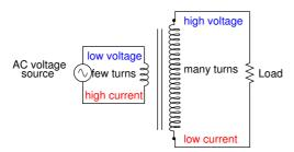
The transformer's ability to step AC voltage up or down with ease gives AC an advantage unmatched by DC in the realm of power distribution. When transmitting electrical power over long distances, it is far more efficient to do so with stepped-up voltages and stepped-down currents
