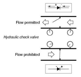
Check valves are essentially pressure-operated devices: they open and allow flow if the pressure across them is of the correct "polarity" to open the gate (in the analogy shown, greater fluid pressure on the right than on the left). If the pressure is of the opposite "polarity," the pressure difference across the check valve will close and hold the gate so that no flow occurs.
