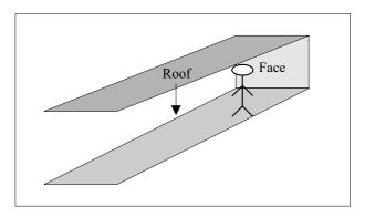
The roof is not one big uniform chunk of rock. Rather it is broken up into smaller chunks. It is assumed that the biggest chunk of rock in the roof has a mass of less than 20 000 kgs therefore each support has to be designed to resist a force related to that mass. The strength of the material (either wood or steel) making up the support is taken into account when working out the minimum required size and thickness of the parts to withstand the force of the roof.
