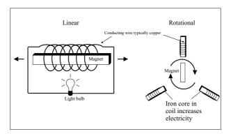
Most power stations produce steam through heat (nuclear reaction or burning fossil fuels), the steam drives a turbine which moves a magnet relative to a coil (the generator like the above but on a much larger scale i.e. bigger magnets, bigger coils, etc), which produces electricity that is transmitted via a power network to our homes. Gas fired plants burn gas directly in a gas turbine to produce the same desired relative motion between permanent magnet and coil.
