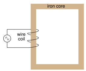
As an inductor, we would expect this iron-core coil to oppose the applied voltage with its inductive reactance, limiting current through the coil as predicted by the equations  $X_L = 2\pi f L$  and I=E/X (or I=E/Z). For the purposes of this example, though, we need to take a more
