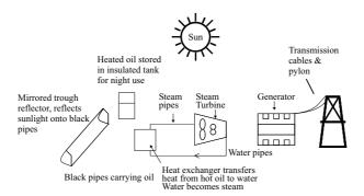
Solar thermal uses the heat of the sun to produce electricity. Sun is concentrated using mirrors. This heat either creates steam which drives a turbine which in turn drives a generator (as per fossil fuel generation), or drives an air engine (engine that uses expanding air to obtain motion) that drives a generator.
