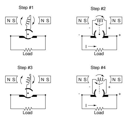
The generator shown above will produce two pulses of voltage per revolution of the shaft, both pulses in the same direction (polarity). In order for a DC generator to produce *constant* voltage, rather than brief pulses of voltage once every 1/2 revolution, there are multiple sets of coils making intermittent contact with the brushes. The diagram shown above is a bit more simplified than what you would see in real life.
