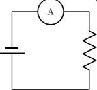
An ohmmeter is an instrument for measuring electrical resistance. The basic ohmmeter can function much like an ammeter. The ohmmeter works by suppling a constant voltage to the resistor and measuring the current flowing through it. The measured current is then converted into a corresponding resistance reading through Ohm's law. One cautionary detail needs to be
