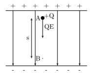
Figure 13.2: A charged particle under the influence of an electric field.
