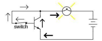
Of course, it may seem pointless to use a transistor in this capacity to control the lamp. After all, we're still using a switch in the circuit, aren't we? If we're still using a switch to control the lamp – if only indirectly – then what's the point of having a transistor to control the current? Why not just go back to our original circuit and use the switch directly to control the lamp current?
