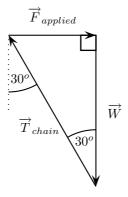
Since the engine is at equilibrium (it is held stationary) the three forces drawn tail-to-head form a closed triangle.
