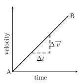
This is the velocity-time graph of a cyclist traveling from A to B at a constant acceleration, i.e. with steadily increasing velocity. The gradient of this graph is just  $\frac{\Delta \vec{v}}{\Delta t}$  - and this is just the expression for acceleration. Because the slope is the same at all points on this graph, the acceleration of the cyclist is constant.
