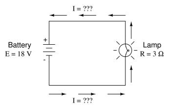
In the above circuit, we know we have a battery voltage of 18 Volts and a lamp resistance of 3  $\Omega$ . Using Ohm's Law to determine current, we get:
