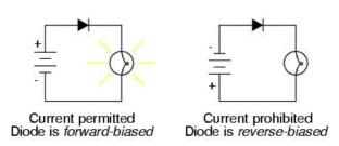
Diode behavior is analogous to the behavior of a hydraulic device called a check valve. A check valve allows fluid flow through it in one direction only:
