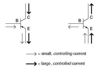
Bipolar transistors are called bipolar because the main flow of electrons through them takes place in two types of semiconductor material: P and N, as the main current goes from emitter to collector (or visa-versa). In other words, two types of charge carriers – electrons and holes – comprise this main current through the transistor.
