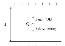
Figure 13.3: An oil drop suspended between oppositely charged parallel plates.
