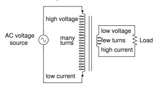
A transformer designed to output more voltage than it takes in across the input coil is called a "step-up" transformer, while one designed to do the opposite is called a "step-down," in reference to the transformation of voltage that takes place. The current through each respective coil, of course, follows the exact opposite proportion.
