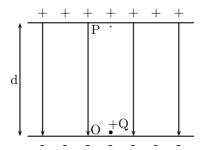
This electric field is uniform so that a charge placed anywhere between the plates will experience the same force. Consider a positive test charge Q placed at point O just off the surface of the negative plate. In order to move it towards the positive plate we have to apply a force QE. The work done in moving the charge from the negative to the positive plate is,
