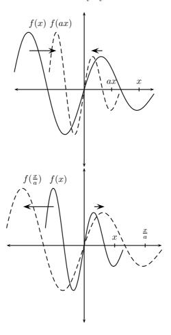
Figure 6.4: Graph of a function with the rescaling  $x \to ax$  and  $x \to \frac{x}{a}$ . Note that these are just a shrinking and stretching in the horizontal axis.
